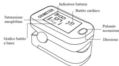
FIG.2 Display a LED
