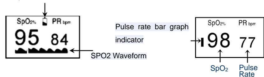
Pulse rate bar graph flashes in relation with pulse rate shown on display.
