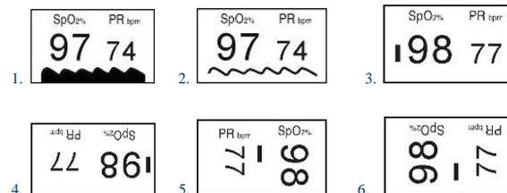
**Brightness regulation.** When you press the power switch for a long time (more than one second), the brightness of the oximeter will be changed by degrees. There are 10 levels on brightness; the default level is level four.
